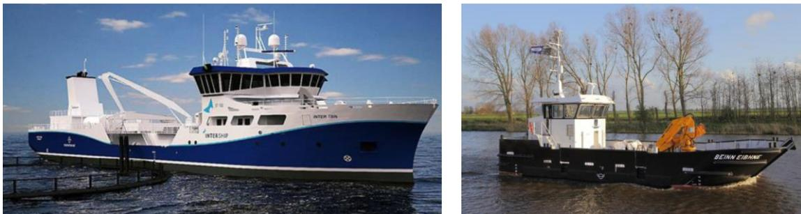
Figure 23: Examples of typical vessels commonly accessing site, a well boat (left) used for freshwater treatments, grading, stocking etc and site-specific workboat (right).
